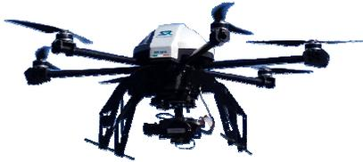
Drone camera Airinov Multispec 4c, rilievi a Vetralla (VT), 2015
